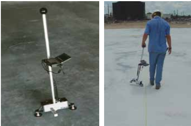
Fig. 5: A Dipstick floor profiler is used to collect flatness and levelness data
